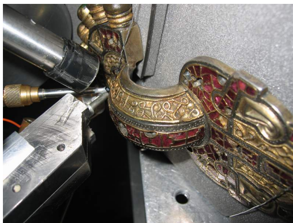
Figure 1: External beam PIXE analysis of garnets set on a 7 th century fibula (Wittislingen, Germany).
